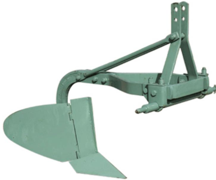
The Implement with the Brand Atespar is SKP type Canal Opener Plough and mounting by three point linkage. Is produced by 10-12-14-16 soc's and with adjustable space. It is usable for Canal opening or Ridging. With the adjusting of soc' s it is good to adjust the spaces as desired. All SKP type ploughs are standart. If it is necessary the Spares might changing easily. All Atespar brand ploughs are checking up after assembling and adjusted at the field for high capacity.
